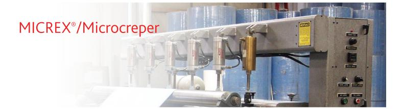
The MICREX Process is a unique, uncomplicated, mechanical technology to impart functional (stretch, extensibility, absorbency, bulk) and esthetic (softness, drape, hand) qualities to a wide range of web structures.
